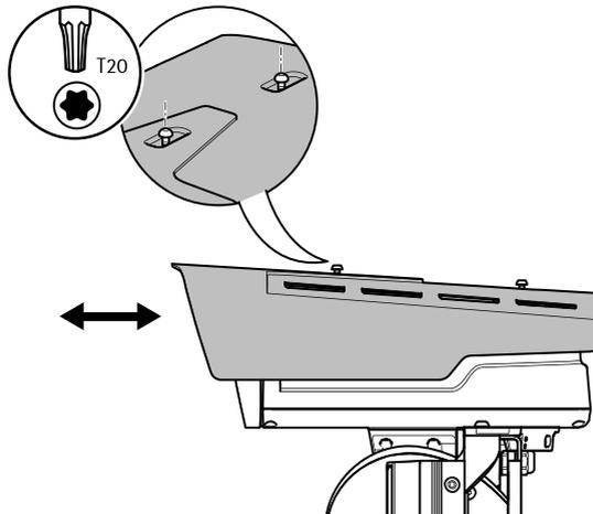
1. Loosen the two weathershield screws.
