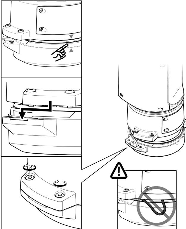
13. Replace the positioning unit on the base unit making sure that the arrows on the two units are aligned.
