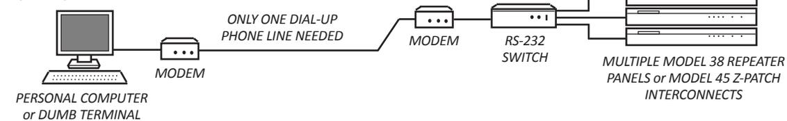
*The best way to control a Model 38 over a phone line is with an RS-232 terminal and a pair of modems. If you have several Model 38s at a common site, use a multiport RS-232 switch so you don't have to obtain multiple phone lines.*
