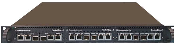
Figure: 1U mTOP™ with 3x PXE100 USB units (MT001 + PXE100)
