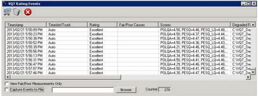
The user may configure a Rating Criteria for all VQT algorithms as well as the additional analytical results. The rating criteria may be configured for Excellent, Good, Fair, and Poor and the results of the rating criteria may be saved to file for post processing viewing.
