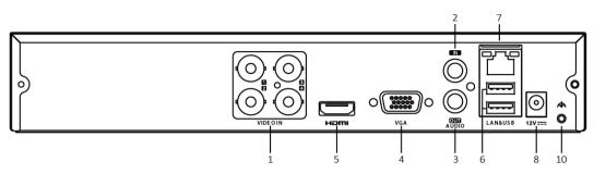
Figure 1-8 Rear Panel of DVR-200Q-K1
