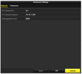
Figure 2-40 Network Configuration of the Camera
