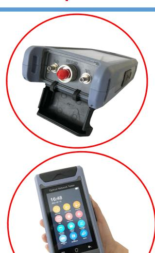
ST3200F series OTDR adopts 4.3 inch capacities touch screen. It integrates 12 functions, such as auto OTDR, expert OTDR, event map, OPM, RJ45 cable tracker, and "computer level" file management to meet various test requirements in different occasions.
